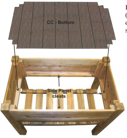
Insert *Bottom CC* (landscaping cloth up) onto *Side Panel Cleats* and secure using 2" screws.
